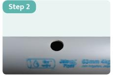
Deburr the hole carefully. Check that no sharp corners are present.
